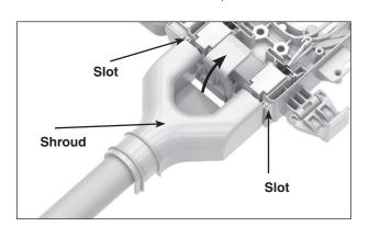
**Step 2:** Secure the shroud to the conduit with the hose clamp provided.
