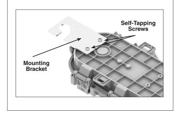
**Step 2:** Hang the closure from the offset ladder bar of the pedestal bracket with the mounting bracket, as shown below.
